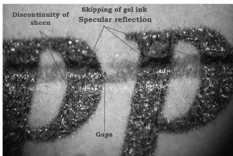
Fig. 9 Characteristics of writing through green gel pen ink observed via stereomicroscope at a 15-degree illumination angle (Saini et al., 2009).
